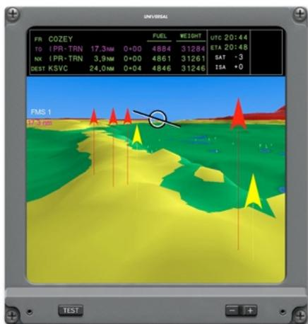
While a Terrain Display is required on Class A TAWS installations, it is technically optional on Class B TAWS installations. However based on working feedback from current TAWS clients and an complete understanding of the system usage and operations under real situations, a display really should be part of **all** TAWS installations. Any added cost will be offset by greatly enhanced situational awareness at all times.
