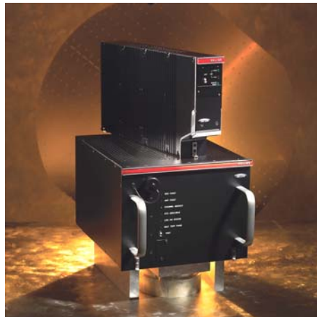
Rockwell Collins SAT-6100B SATCOM and HST 2110B. First certified in late 2008, this new Rockwell combination offers a range of SwiftBroadband (SBB) functionality along with automatic fallback to Swift 64 when out of SBB's coverage.
