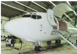
The distinctive up swinging cargo door of the 737-200C – the reason that this aircraft is able to service Falconbridge as it does. (photo by MC2)
