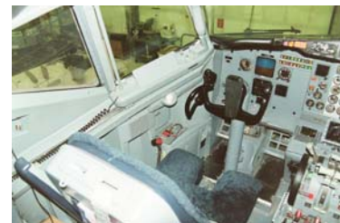
New switching and annunciation panels were developed and located to effectively reduce pilot workload and increase situational awareness. (photo by MC2)
